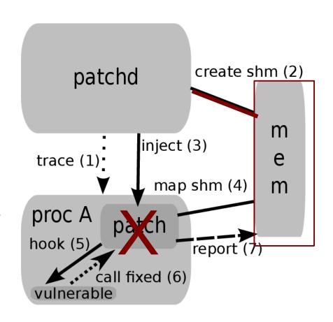
Enables scalable testing of patches in the field
